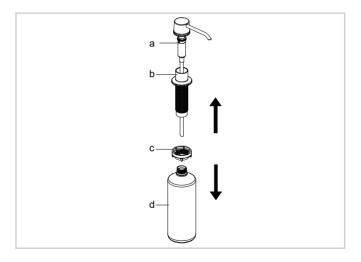
Install dispenser base (b) attached into the hole in the countertop. Re-install mounting nut (c) on the dispenser base (b) from underneath the countertop. Tighten mounting nut (c) by hand.
